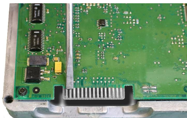
Figure 2 - Cleaning the clear lacquer
