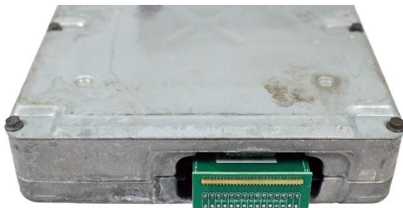
Figure 5 Installing the chip
